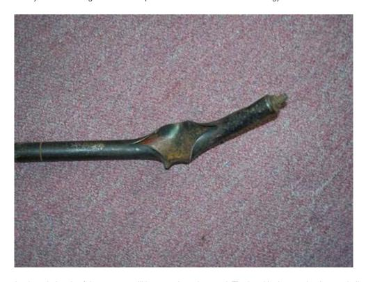
(1) Note the threaded ends of the strut are still intact and not damaged. The bend in the strut leads us to believe it is possible that it expanded while still fixed to the unit and was under excessive pressure with the cylinder wall seam failing as the weakest point.
