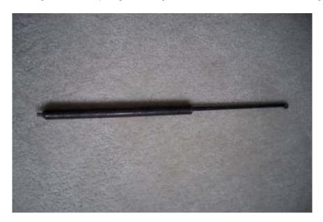
(3) The second cylinder rocketed and imbedded in the wall. The cylinder, the piston rod, and the threaded connections at each end are all intact. The rod moves freely, without resistance, for the length of the throw of the cylinder, but it feels as if the seal at the end of the rod inside the cylinder was damaged and no longer sealed.
