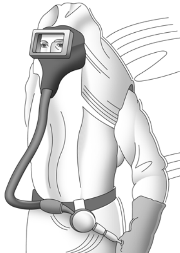
Tight-fitting Abrasive Blasting Respirator Continuous flow APF=25/1,000* SAR Full Facepiece Needs to be fit tested**
